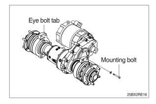
Remove 5 mounting bolts fixing the motor
