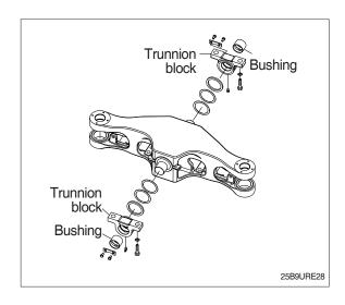
(2) When installing trunnion block, make sure the space at the back in under 0.5 mm when it was pushed completely.
