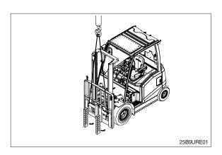
② While supporting lift chains, remove the split pin and nuts from the chain anchor.
